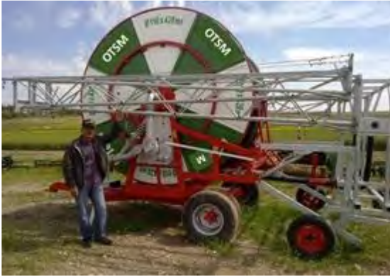
Figure 1. Hose reel irrigation machine with a boom
